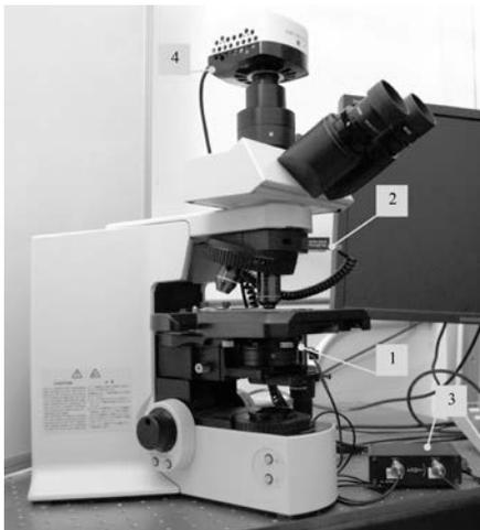
OI-DIC components installed on upright microscope Olympus BX61. (1) Condenser-side beam-shearing DIC assembly; (2) objective-side beam-shearing DIC assembly; (3) Arcoptix USB LC-cell controller; (4) Lumenera monochromatic CCD camera.
