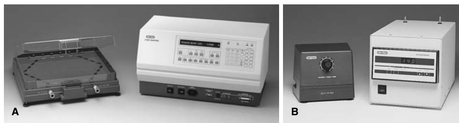
Fig. 1.3. A. The complete CHEF Mapper XA chiller system, with chamber and power module, and B. variable speed pump and Cooling Module.
