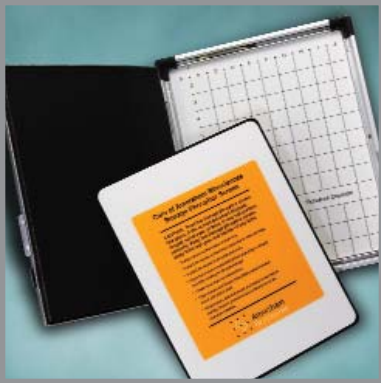
Fig 4. Storage phosphor screens are available in several different formats and sequencing gel sizes. With proper care, storage phosphor screens last indefinitely, regardless of how often they're used. A ten minute exposure to visible light prepares the screen for reuse.
