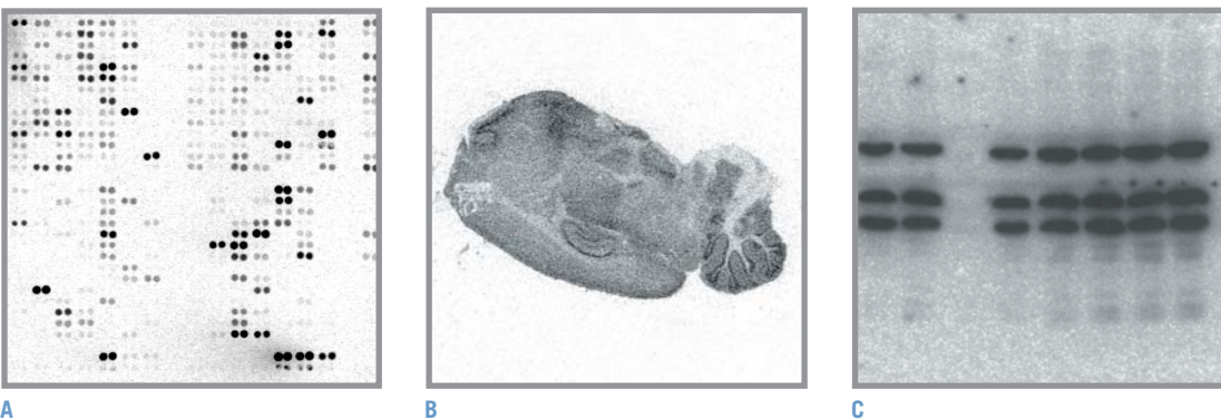
Fig 7. A) Macroarray imaging of small or large format cDNA arrays is easily performed for gene expression profiling. B) Tritium-labeled samples can be imaged with tritium screens. Storm system's 50- \mu m pixel resolution enables visualization of even the fine detail of tissue structure. C) Southern, Northern, Western, and other radiolabeled blotting assays produce images on storage phosphor screens 10–100 times faster than with film. And Storm imager lets you choose any radioisotope (or use nonradioactive chemifluorescence) for blotting applications. Courtesy of Christopher Hug, Dept. of Cell Biology, Washington University Medical School, St. Louis, Missouri, U.S.A.
