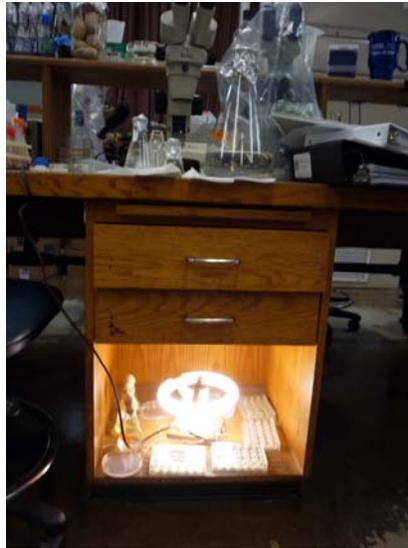
Figure 1. The experimental setup for growing of *Synechocystis*. All reactors and assay were adjacent to the fluorescent light source.
