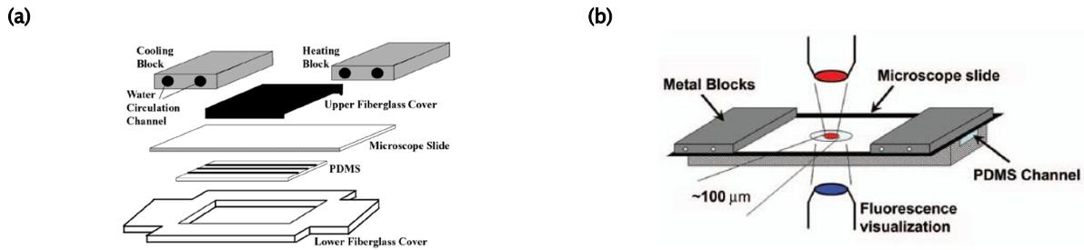
**Figure 1.** Examples of experimental systems for thermotaxis assays. (a) A set of narrow channels (0.07x0.002 cm), 3 cm long, microfabricated with polydimethyl-siloxane (PDMS; Salman *et al.* 2006). (b) Thin channels (700x20μm) microfabricated in PDMS and covered by 1-mm-thick glass microscope slide. An infrared laser ( $\lambda=1,480\text{nm}$ ) is focused into the channel through the glass slide using a 32x objective (Salman and Libchaber 2007).
