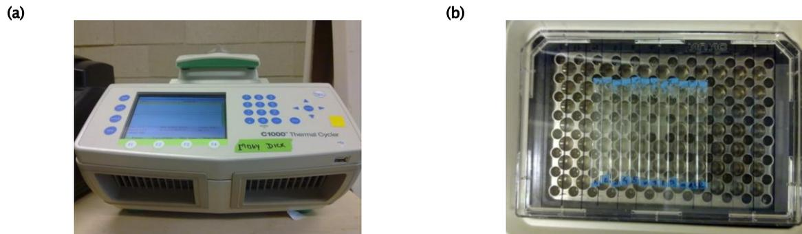
**Figure 3.** Experimental setup for a capillary assay in a gradient thermocycler. (a) BioRad C1000™ gradient thermocycler. (b) Capillaries incubated along the temperature gradient.
