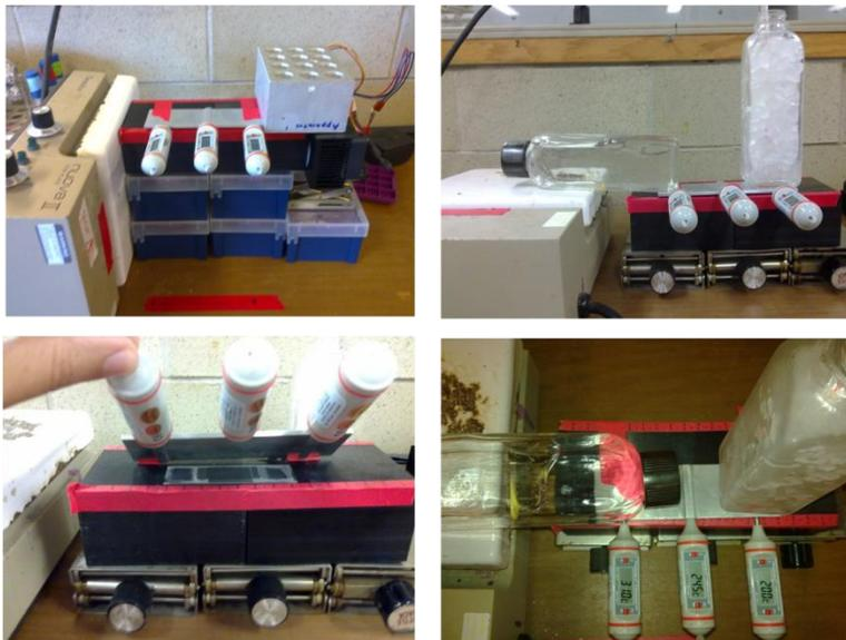
**Figure 7.** Process of development of a small aluminum temperature gradient block for a microchamber assay.
