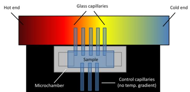
**Figure 2.** Idealized setup for a capillary assay in an aluminum temperature gradient block.
