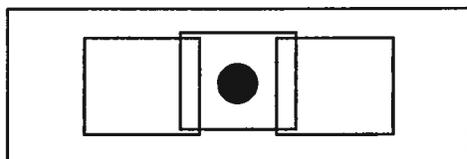
The space between the middle coverslip and the slide was flooded with washed cell suspensions in SW media base (.01% glycerol can be added if the cells lose their motility
