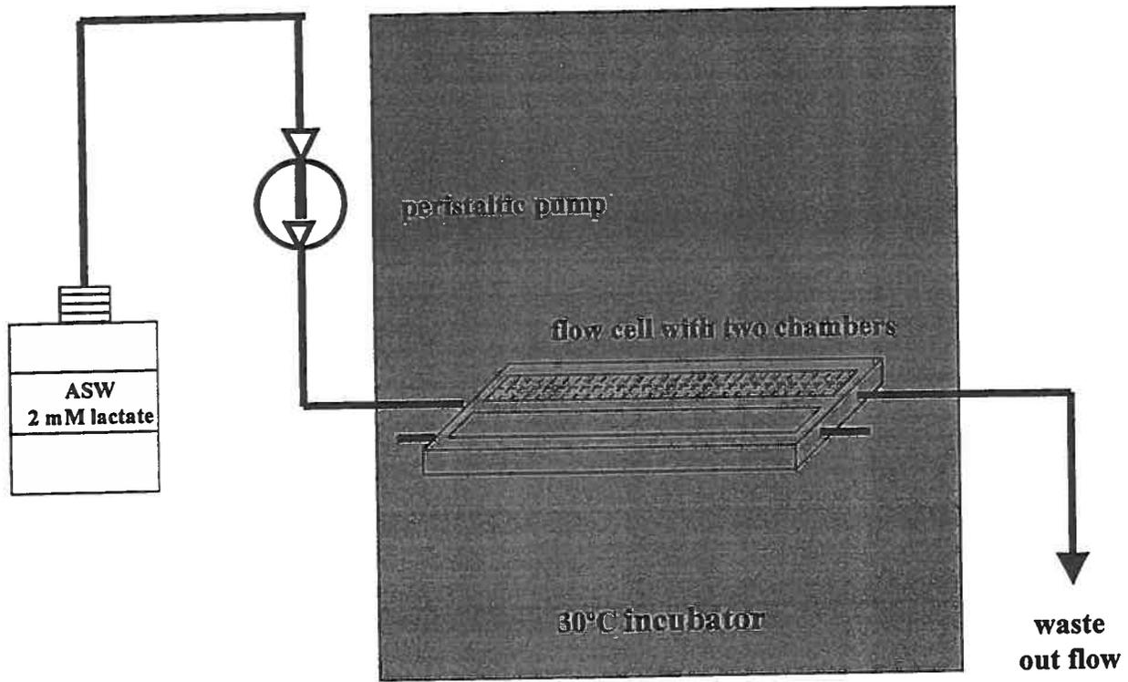
Fig.02: Schematic representation of the experimental design showing peristaltic pump and laminar flow cell. The cell was run with ASW medium and 2 mM lactate.
