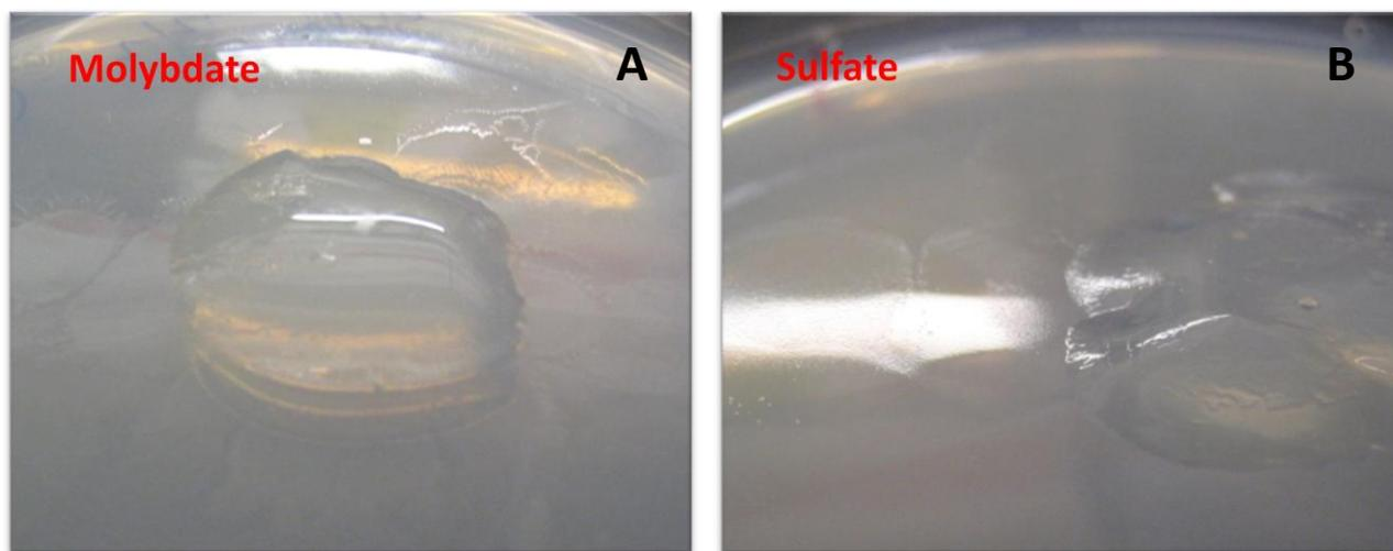
**Figure 3.** Test for presence of sulfate reducing bacteria with molybdate (A) added to inhibit the sulfate reducers and sulfate (B) is added as control.
