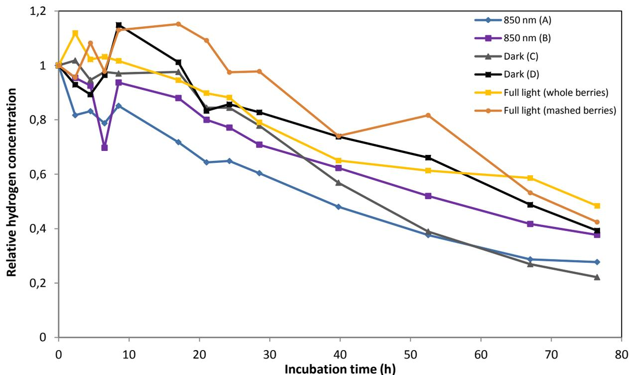
**Figure 6.** Relative hydrogen consumption as function of time in all six microcosms. All values have been corrected for volume removed at each sampling point.
