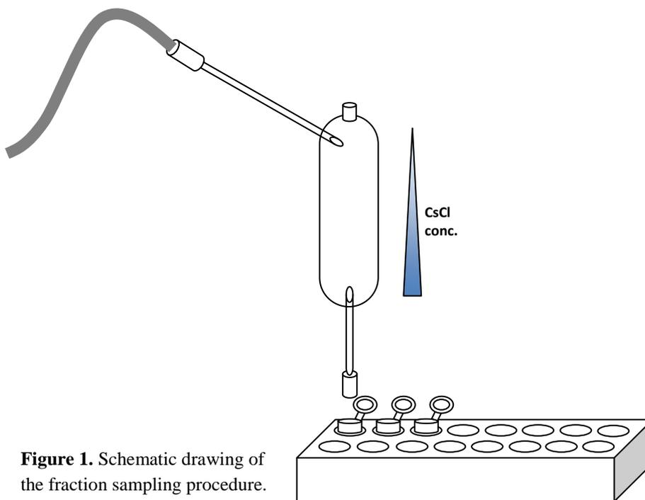
**Figure 1.** Schematic drawing of the fraction sampling procedure.
