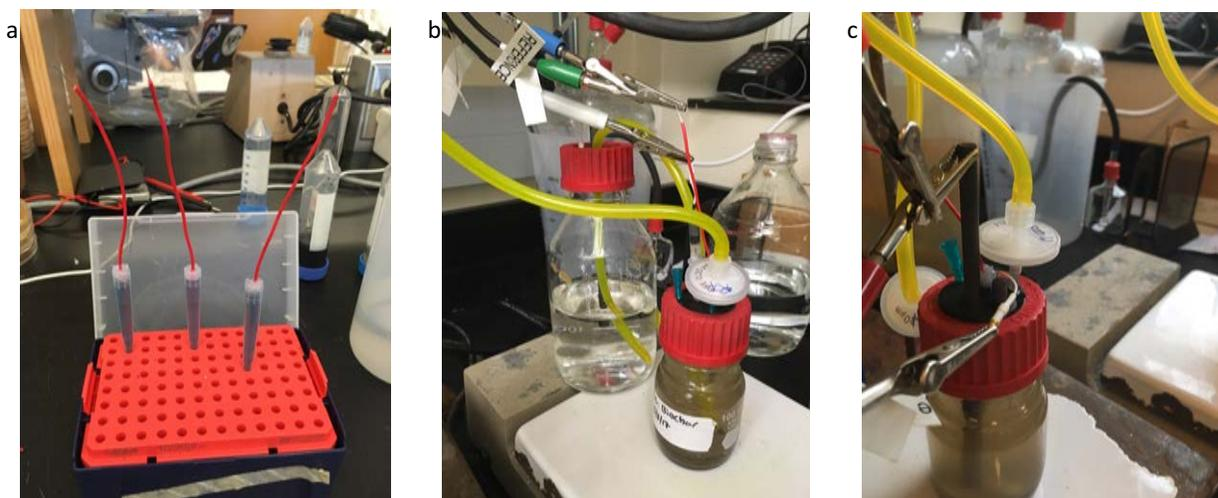
Figure 1: a) biochar anodes. b) succinate MFC with biochar anode using both anaerobic (small) and aerobic (big) bottles. c) Acetate MFC with biochar anode in one anaerobic bottle.
