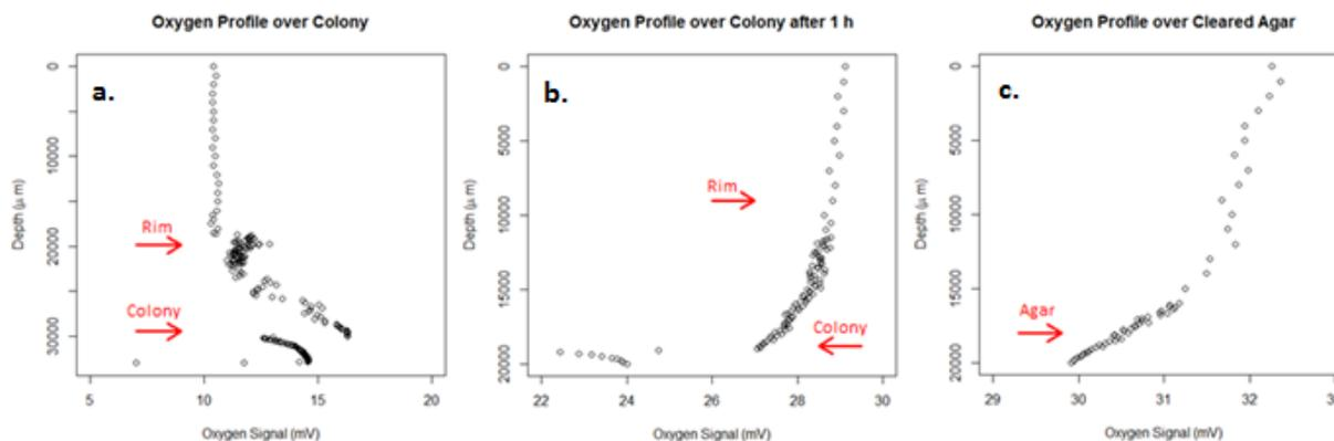
Figure 3: Oxygen profiles over MnO<sub>2</sub> pie plate with white, circular Mn(IV) reducing isolate. Oxygen increases from ambient levels around colony within 20 min of opening the dish (a), whereas oxygen levels continually decline over MnO<sub>2</sub> clearings in the agar (b) or over a colony after 1 h of the dish being opened (c). Axes are NOT identical.
