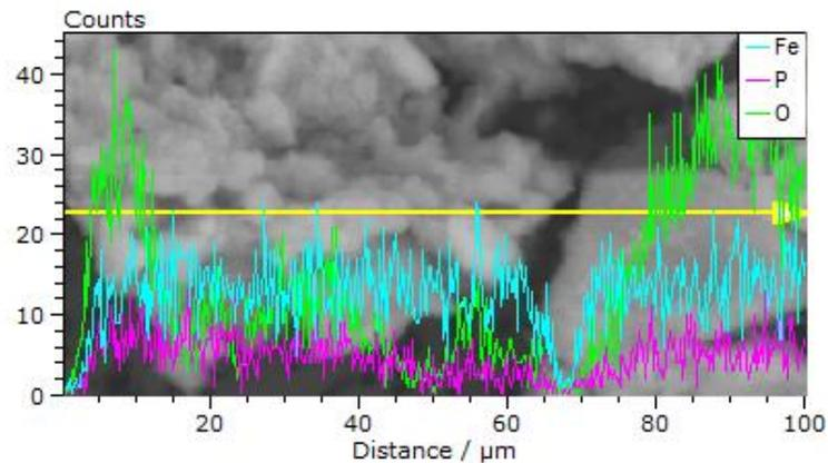
Figure 8: Transect along minerals from School St. + dextrose enrichment. Fe:O ratio varies between particles, meaning that  $Fe_2O_3$  reduction occurred but was not complete despite completely black (to the unaided eye) solids.
