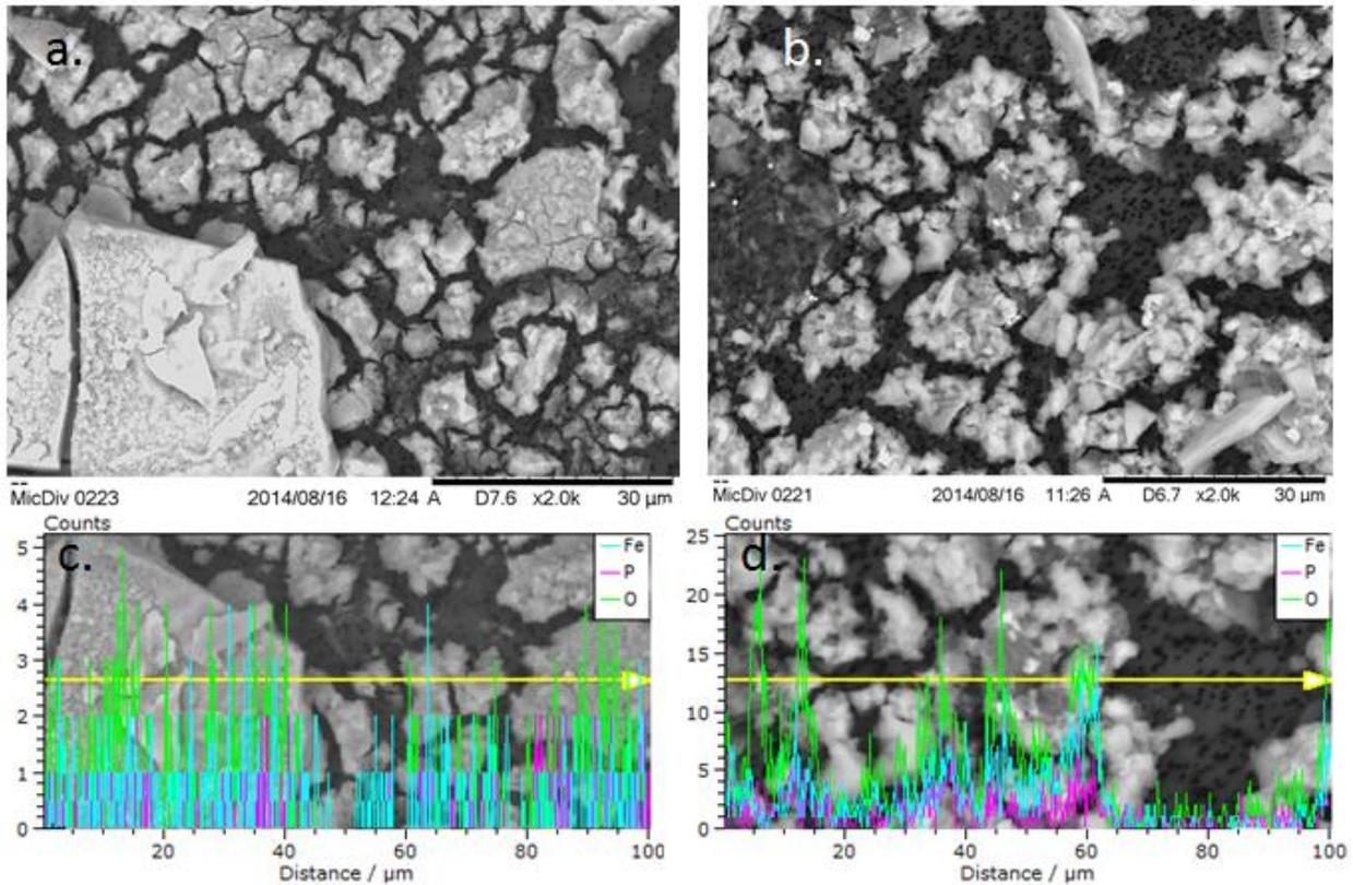
Figure 7: Poorly crystalline iron(III) oxides (a) and iron(II) oxides (b) viewed by SEM with transects depicting Fe, P and O content in the Fe(III) (c) and Fe(II,III) minerals (d), analyzed using EDS. PCIO was taken from an uninoculated control jar. Reduced iron oxides were taken from the School St. + dextrose enrichment 10 days after inoculation.
