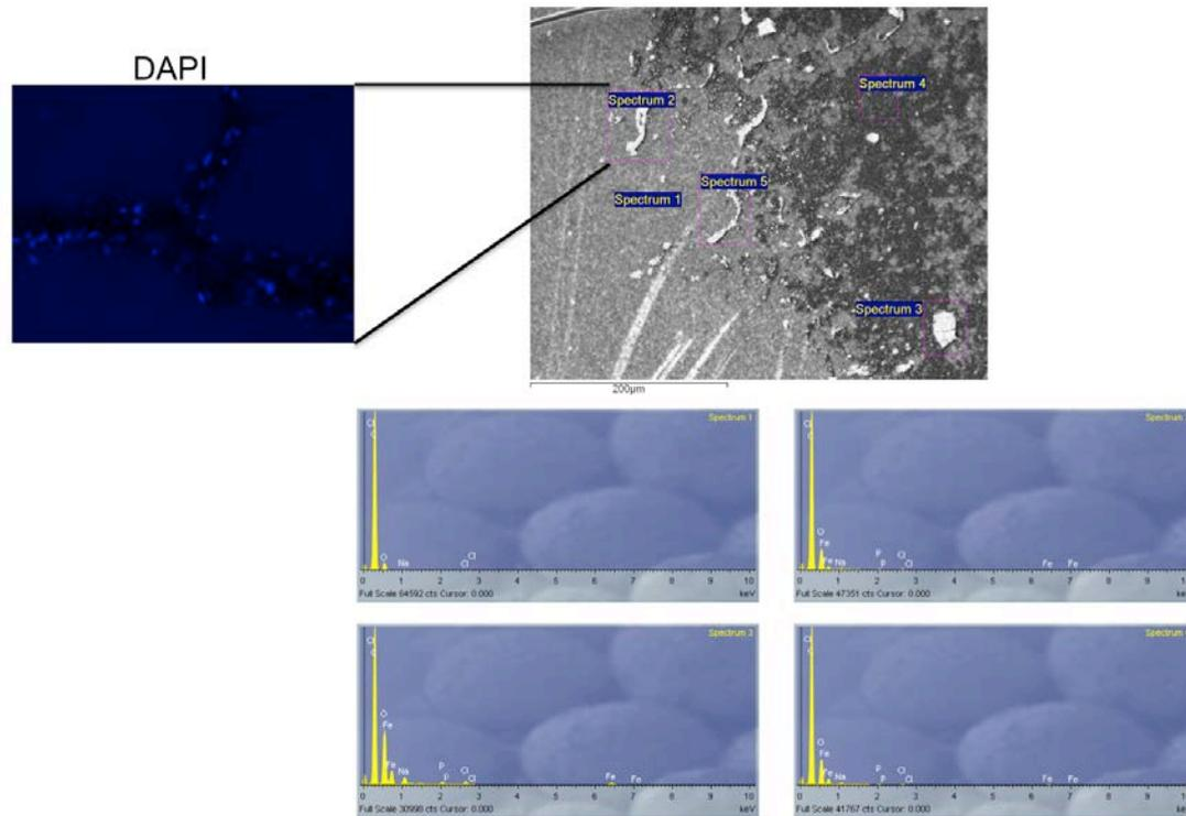
**Figure 6: Energy-dispersive X-ray spectroscopy (EDS).** The EDS reveals that the filamentous superstructure form by the FRM were consist of main carbon compound instead of iron.
