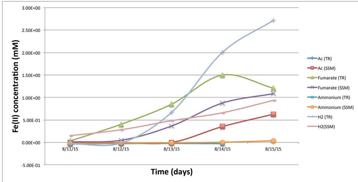
**Figure 3: Fe<sup>2+</sup> concentration in the secondary enrichment culture.** The increase in Fe<sup>2+</sup> is more prominent in the hydrogen enrichment while the fumarate enrichment has the highest Fe<sup>2+</sup> production rate
