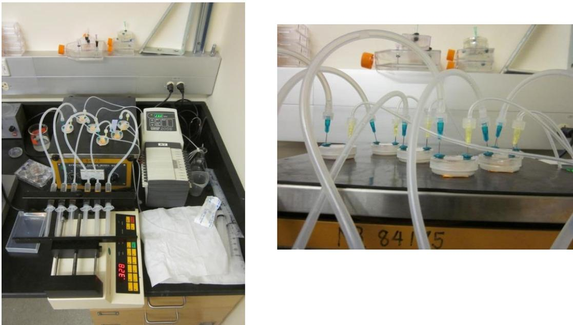
Figure 1. Flow chamber set up for 35 mm MatTek dishes.
