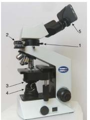
Polychromatic polscope for field studies. (1) microscope Olympus CX21; (2) polychromatic polarization state generator; (3) polarizer; (4) mirror unit CH20MM; (5) iPhone 6S with adapter.
