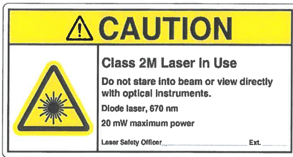
Figure 1. Sample warning sign for Class 2, Class 2M, and Class 3R lasers. From ANSI Z36.1-2014 (Figure 1a).
