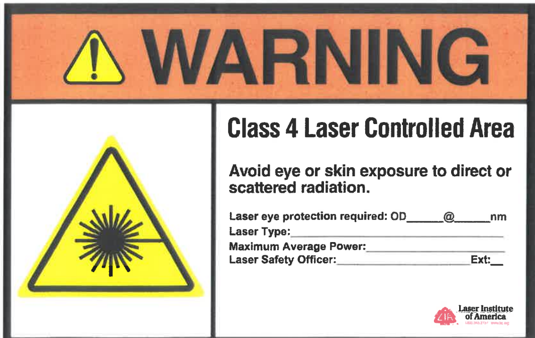
Figure 3. Sample warning sign for Class 4 Laser Controlled Area. Adapted from ANSI Z36.1-2014 (Figure 1c).
